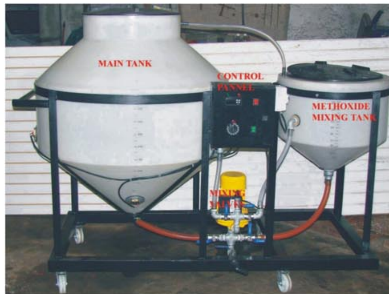
BP400 BIO-DIESEL REATOR
